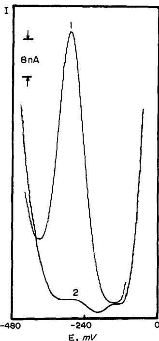
Fig. 5. Polarograms of uranium mineral extracts, in chloroform in the presence of 0.75M PP/0.25M P as supporting electrolyte (1) decomposed with HNO 3 , (2) decomposed with HNO 3 + HF V = 10 mV f = 75 Hz t = 1 sec.
